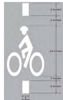
MUTCD Bicycle Detector Pavement Marking
